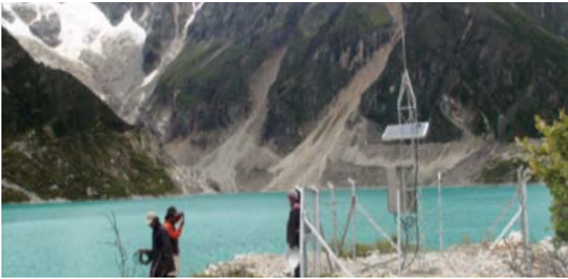
Figure 11: Automated early warning systems are installed to give downstream population a head start to evacuate the disaster zone.
